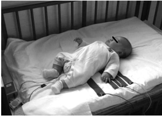
Fig. 1. An image of a subject (#2) lying supine on the bed-sheet electrode unit. Black striped rectangles are fabric electrodes. Three wire leads from the electrodes are connected to the developed signal extraction device. Wires from the crotch portion are the lead for reference ECG measurement.
