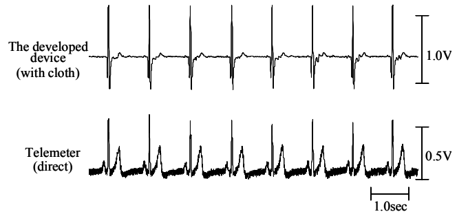
Fig.6. ECG recordings using the developed device with cloth (top) and using commercial telemeter system without cloth (bottom)
