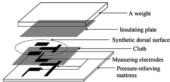
Fig. 5. Experimental setup for measuring frequency-gain characteristics of the developed system while a cotton cloth was inserted
