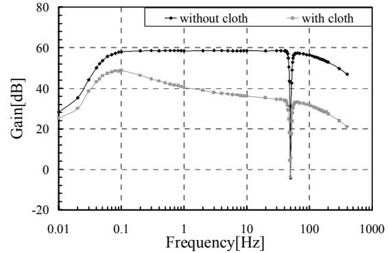
Fig. 6. Frequency response obtained without cloth and with an inserted cotton sheet subjected to 569 Pa pressure. Black rhombus plots show the original frequency-gain response of the developed system without an inserted cloth and grey square plots show the one obtained with the cloth.
