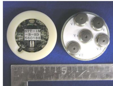
Fig. 3. An Image of the developed wireless electrode for Laplacian EMG measurement. The left is top view and the right is bottom view.
